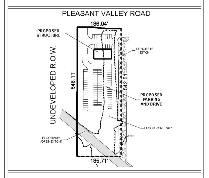
The site is located on the South side of Pleasant Valley Road, 350' West of Delmar Drive. The plan illustrates the existing drainage and proposed structures.
