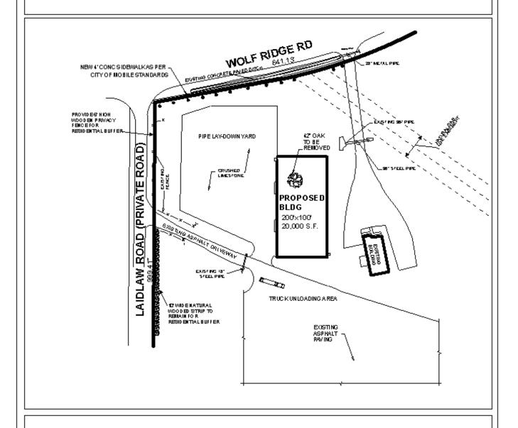
The site is located on the Southeast corner of Wolf Ridge Road and Laidlaw Lane (private street). The plan illustrates the existing structure, drives, and parking, along with the proposed building and sidewalk location.
