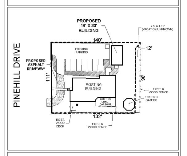
The site is located on the East side of Pinehill Drive, 160' South of Airport Boulevard. The plan illustrates the existing and proposed structures and paving.
