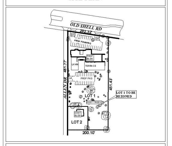
The site plan illustrates the proposed building, parking, curb cuts, lot configuration, along with existing trees and curb cuts.
