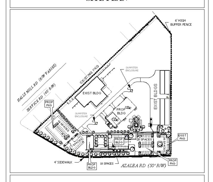
The site plan illustrates existing buildings, parking, dumpster enclosures, buffer fence, and proposed buildings and parking.
