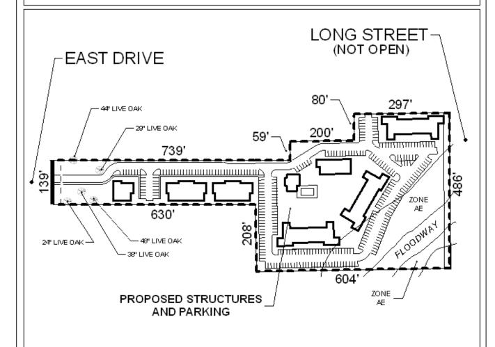
The site is located on the East side of East Drive, 900' South of Old Shell Road, extending to the West side of Long Street, 600' South of Old Shell Road. The plan illustrates the proposed structures and parking as well as the existing trees and floodzones.
