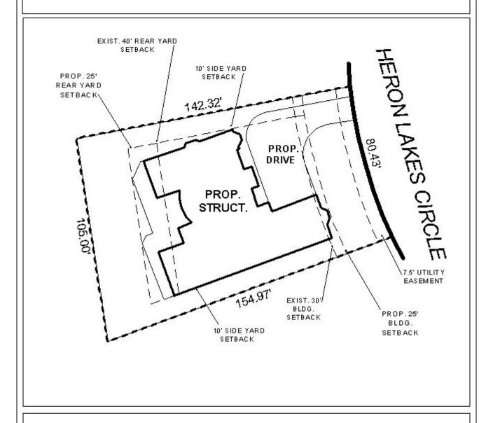
The site is located on the West side of Heron Lakes Circle, 75' South of Heron Lakes Drive. The plan illustrates the existing and proposed setbacks along with the proprosed structure and drive.
