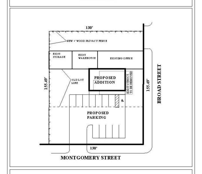
The site is located on the Northwest corner of Broad Street and Montgomery Street. The plan illustrates the existing structures, along with the proposed addition and parking.
