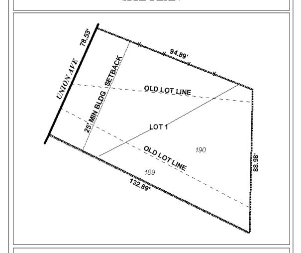
The site plan illustrates the existing lot lines and fencing along with the proposed lot configuration and setbacks.
