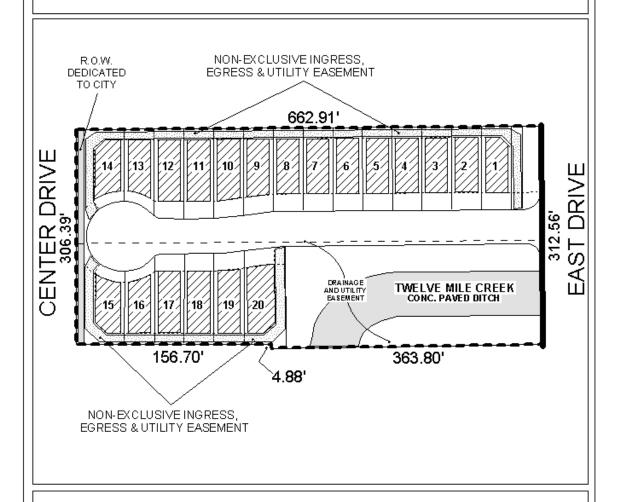
The site is located on the West side of East Drive, 3/10 mile South of Old Shell Road, extending to the East side of Center Drive. The plan illustrates the proposed structures, easements and drives.
