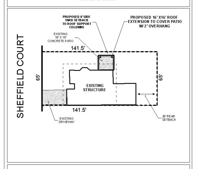
The site is located on the East side of Sheffield Court, 215' South of Japonica Lane. The plan illustrates the existing structure, proposed structure and building limits.
