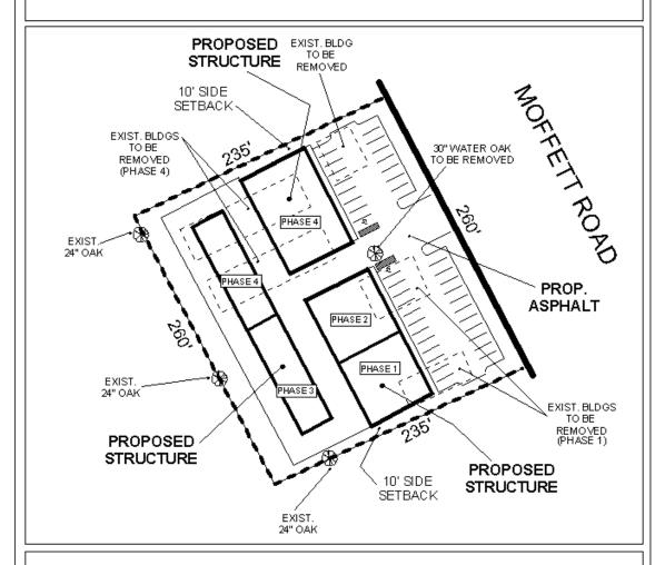
The site is located on the South side of Moffett Road at Pine Grove Avenue. The plan illustrates the existing and proposed structures, setbacks, paving and trees.
