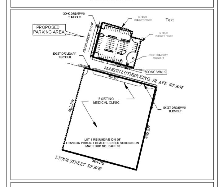
The site plan illustrates parking, concrete driveway turnouts, and concrete walk.
