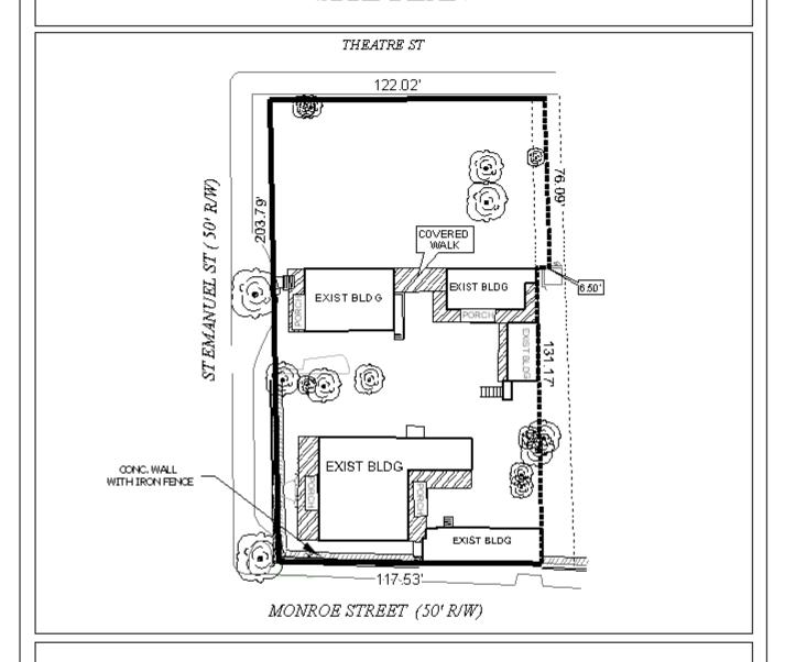
The site plan illustrates the existing buildings, concrete/brick walls, and fence.
