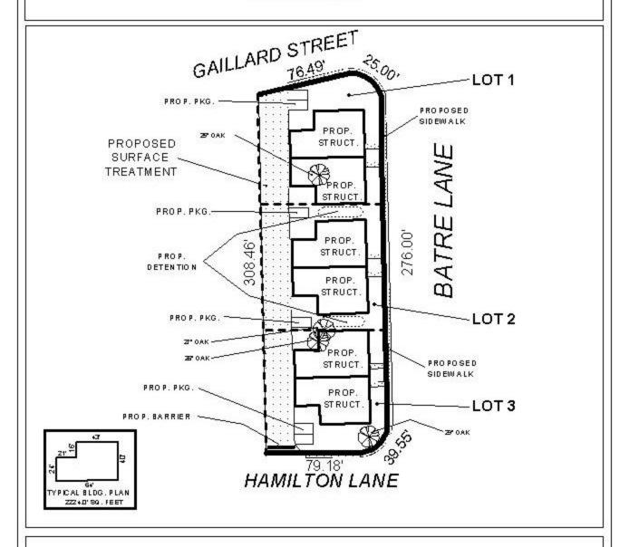
The site is located on the West side of Batre Lane, extending fron the North side of Hamilton Lane to the South side of Gaillard Street. The plan illustrates the proposed structures and paving. Existing trees larger than 24" diameter are also shown.
