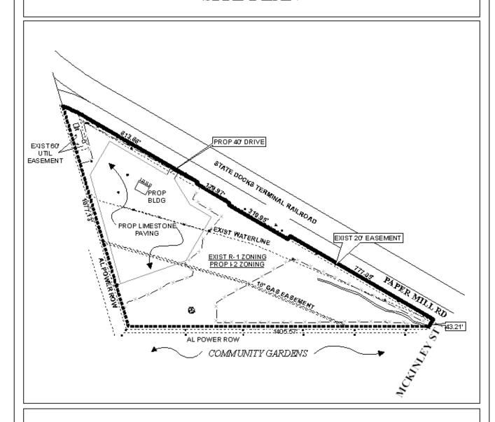
The site plan illustrates the existing utilities and easements, proposed building, drive, and proposed paving area
