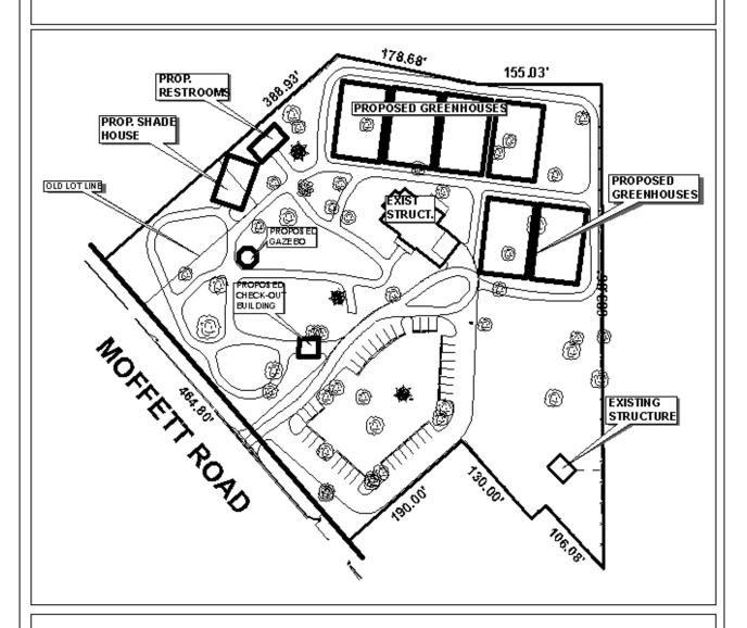
The site is located on the North side of Moffett Road, 225' East of Colonial Circle South. The plan illustrates the existing buildings and drive, along with the proposed structures and drive.
