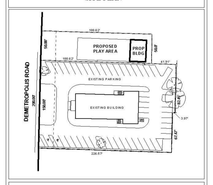
The site is located on the East side of Demetropolis Road, 250' South of Troy Lane. The plan illustrates the existing structure and parking, along with the proposed building and play area.
