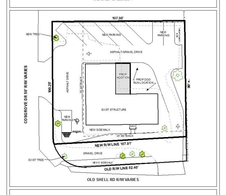
The site plan illustrates the exiting building, proposed addition, new parking, new and exisiting trees, and setback.
