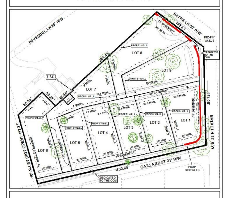
The site plan illustrates the proposed lots, setbacks, easements, and proposed masonry walls.
