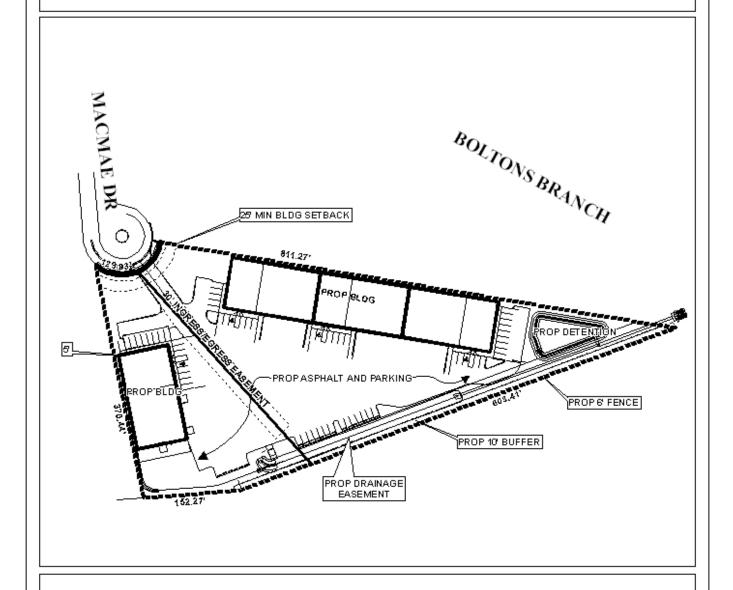
The site plan illustrates the proposed buildings, parking, drainage, and buffer strip
