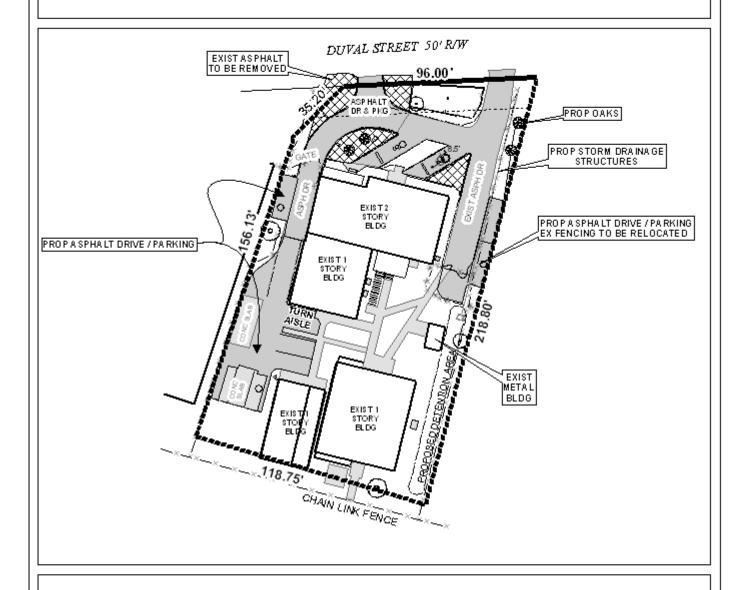
The site plan illustrates the existing buildings, drives, proposed drives, and proposed parking
