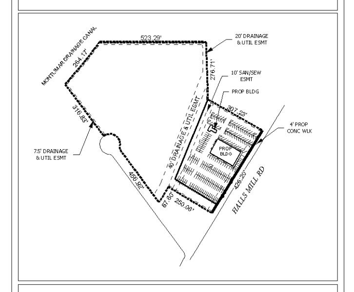
The site plan illustrates proposed parking, buildings, easements, and concrete walk.
