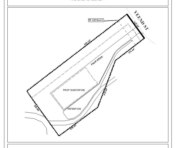
The site plan illustrates the proposed, drive, fencing, and electrical substation
