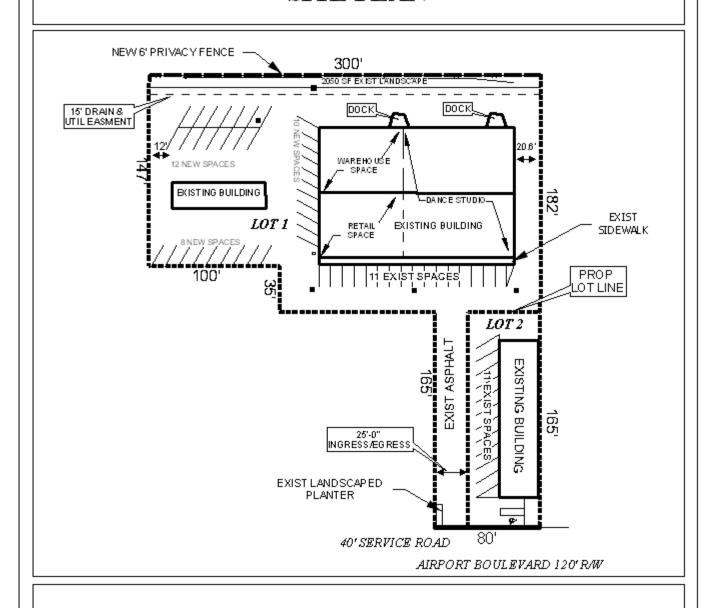
Existing Buildings, drainage and utility easments, asphalt, and proposed lot lines are illustrated in the site plan.
