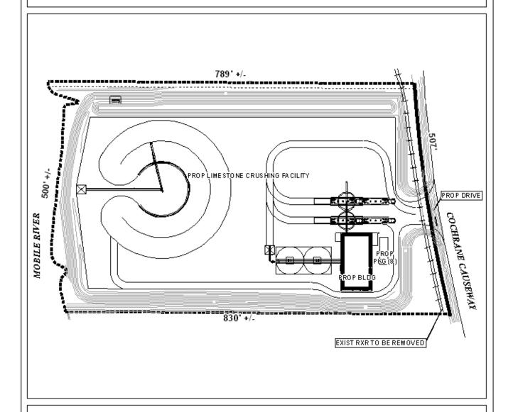
The site plan illustrates the proposed limestone crushing facility
