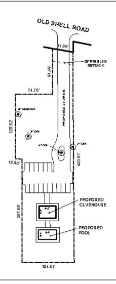
The site is located on the South side of Old Shell Road, 150' East of Wilroh Drive East. The plan illustrates the proposed building, parking, and pool.
