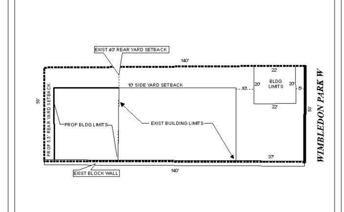
The site plan illustrates the existing building limits, setbacks, and proposed building limits
