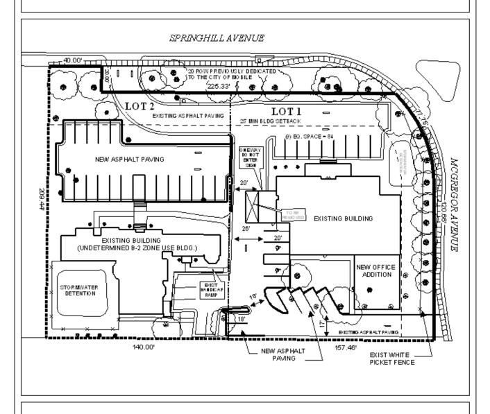
The site plan illustrates the new office addition, new paving, parking, drives and setbacks.
