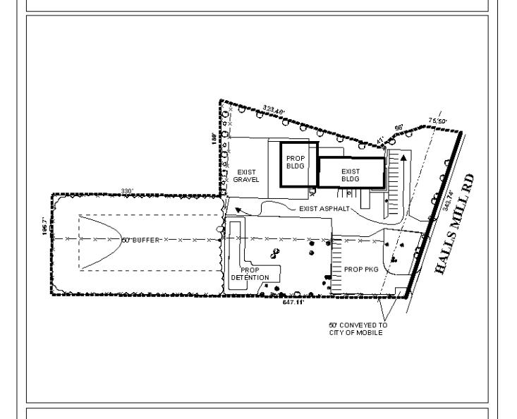
The site plan illustrates the existing building, parking, proposed building addition and proposed parking
