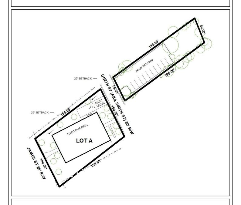
The site plan illustrates the existing building, existing drive, proposed parking, and setbacks.
