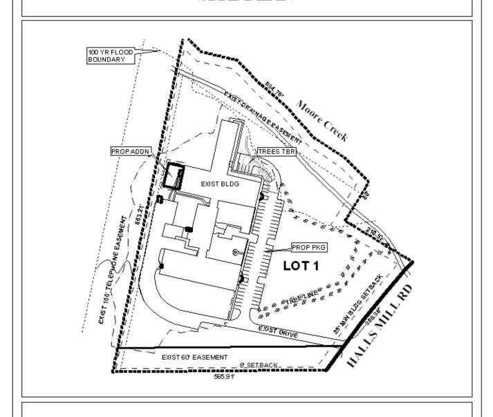
The site plan illustrates the existing building, proposed building additions, and proposed parking expansion
