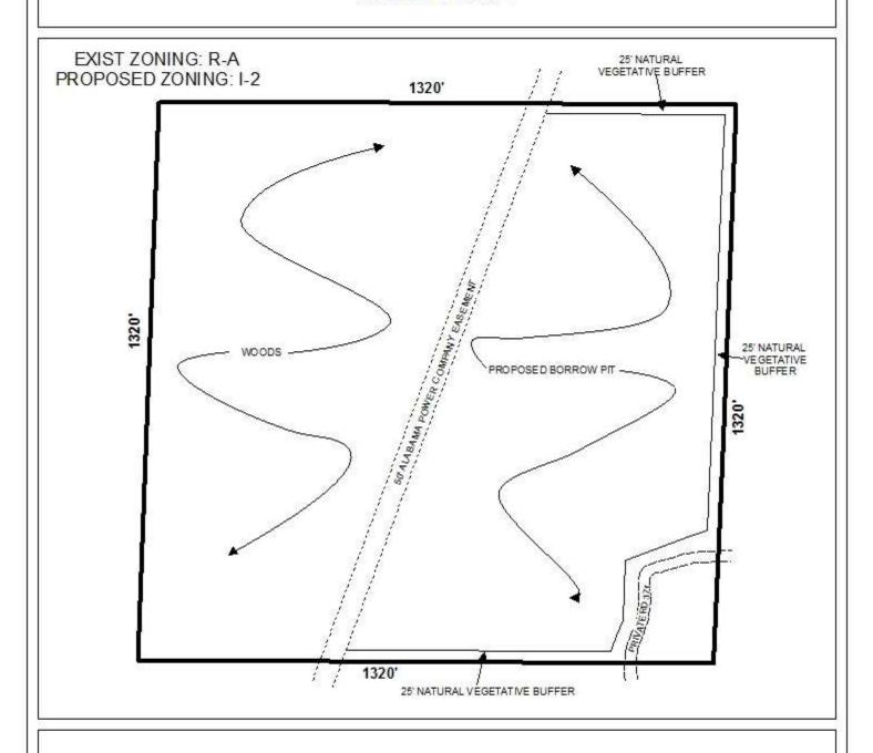
The site plan illustrates the wooded area, proposed borrow pit, easement, and vegetation buffer.
