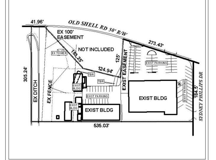
South side of Old Shell Road, 30' East of I-65 Service Road North, the site plan illustrates the existing drainage, utility, and proposed access easements, existing buildings, parking, and fencing
