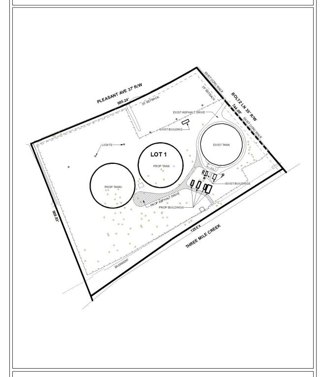
The site plan illustrates the existing tank, existing asphalt drive, existing buildings, easement, setbacks, proposed tanks, and proposed buildings.
