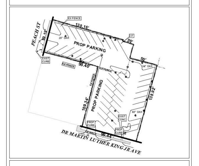
The site plan illustrates the proposed parking spaces, proposed curb cuts, existing fencing, concrete, curb cuts, sidwalks, and trees.
