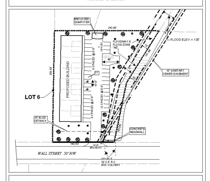
The site plan illustrates the proposed building, easements, culverts, and drives.
