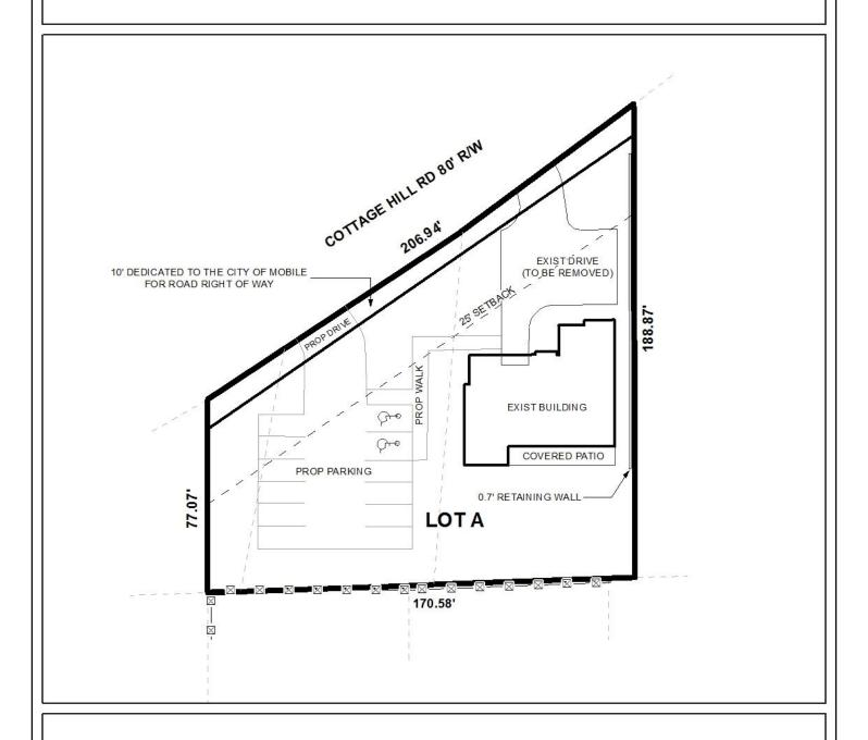
The site plan illustrates the existing building, existing drive, proposed drive, proposed parking, and setbacks.
