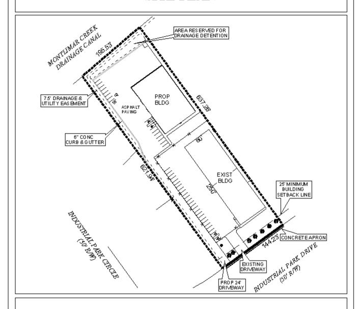
The site plan illustrates the proposed building, parking, proposed drive, setbacks, and easements.
