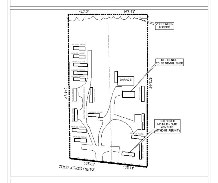
The site plan shows existing and proposed mobile homes, drive, and building to be demolished.
