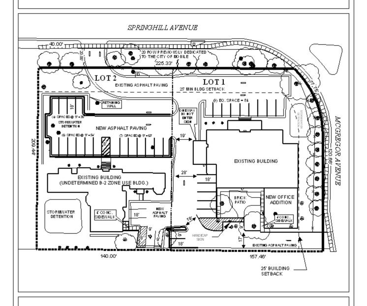
The site plan illustrates the new office addition, new paving, parking, drives and setbacks.
