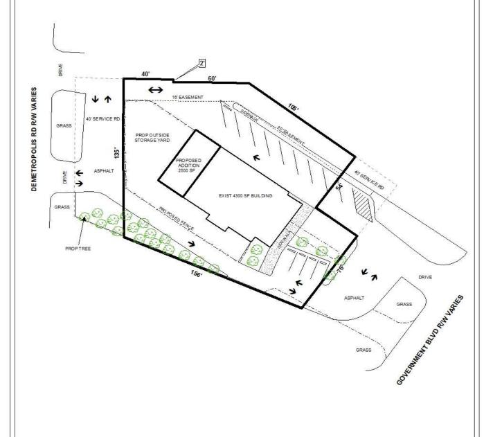
The site plan illustrates the proposed addition, exist building, proposed trees and fence, exist easements, and drives,
