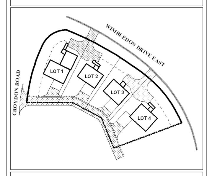
This site plan illustrates existing lot configuration. See detail site plan for sidewalk cross section.
