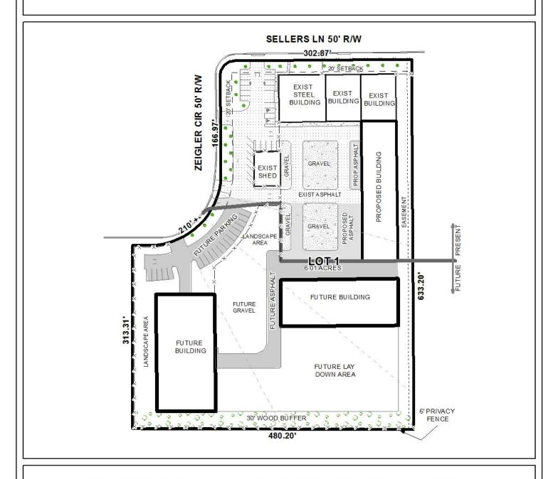
The site plan illustrates the existing and proposed surfaces, and existing and proposed buildings.
