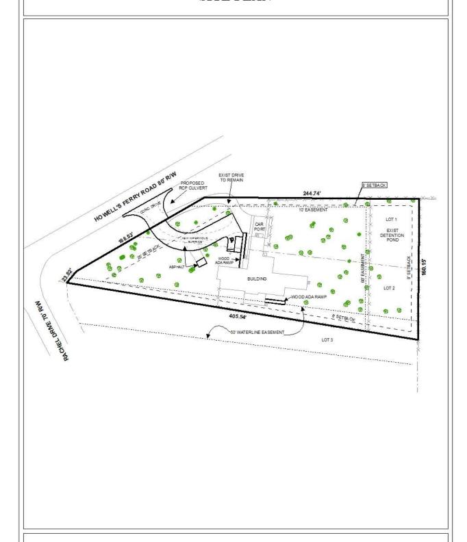
The site plan illustrates the setbacks, easements, new impervious surface, and driveways.
