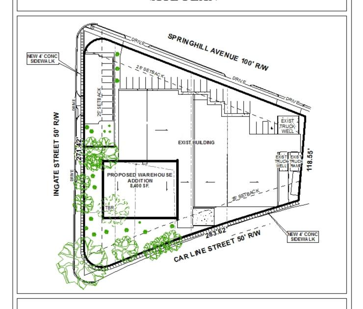
The site plan illustrates the existing building, proposed additions, new sidewalks, and existing trees.
