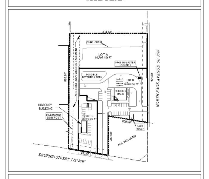
The site plan illustrates the existing and proposed buildings, parking, and access easement.
