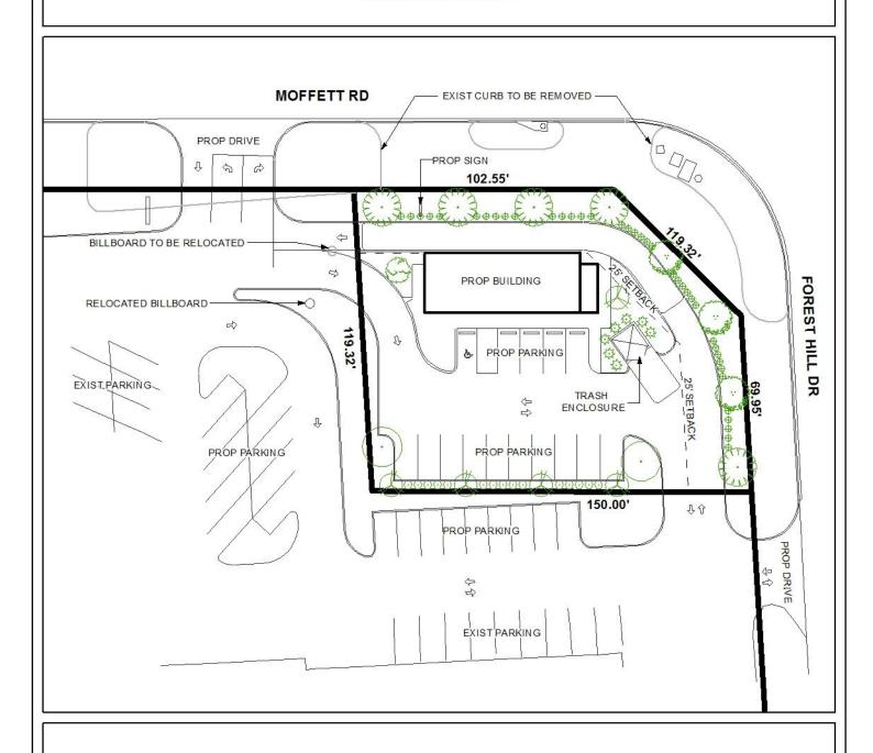
The site plan illustrates the existing parking, proposed building, proposed parking, proposed drives, and setbacks.
