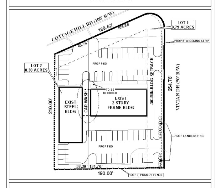
The site plan illustrates the existing buildings, proposed parking, and proposed building to be removed
