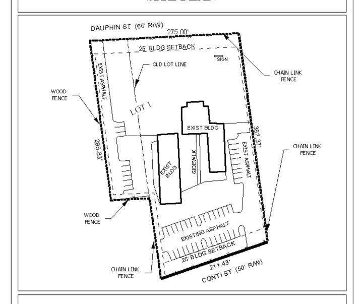
The site plan illustrates existing buildings, asphalt, parking, sidewalk, fences and setbacks.
